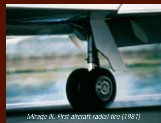
Mirage III. First aircraft radial tire (1981)
